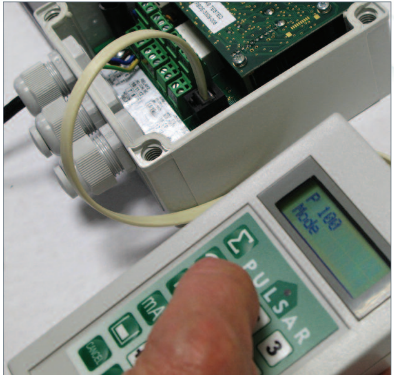
REMOVABLE HAND-HELD PROGRAMMING UNIT CONNECTED TO BLACKBOX
